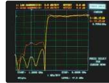
The Return Loss measurement of a low pass filter is grossly distorted when high harmonics are present. When the source's fundamental frequency passes 2 GHz, the second harmonic (at 4 GHz) enters the lowpass filter's reject band; thus, 100% of the second harmonic power is reflected back toward the source. Thus, the reflected harmonic power is measured and then erroneously displayed as the return loss characteristic between 2 and 4 GHz.
