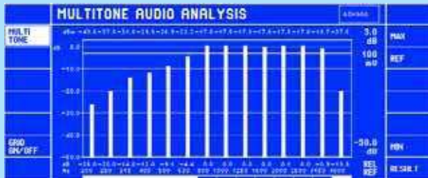
The audio measurement option CMD-B44 is capable of generating and analyzing up to 14 freely configurable tones in about 1 second. Measurements in absolute and relative mode are possible
