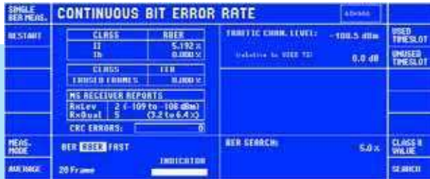
The BER search function allows the absolute sensitivity of a mobile to be determined
