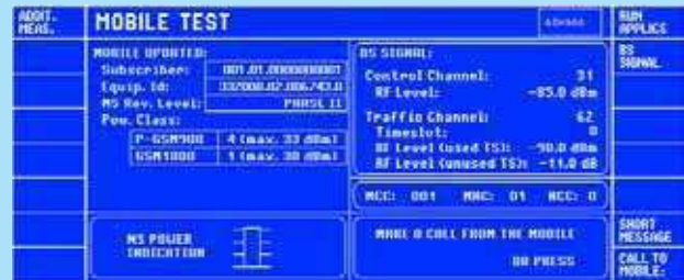
After location update, it is indicated whether a mobile is a dual-band version. For realistic simulation of the real networks, the CMD-U20 offers the option to have the BCCH present in either band during dual-band simulation
