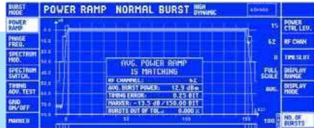
The full dynamic range (>72 dB) of a GSM normal and access burst can be verified with the CMD-B42 option
