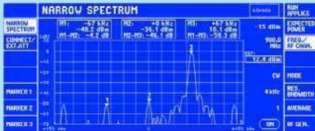
The narrowband spectrum analyzer option CMD-K43 is used to determine the I/Q modulator balance by measuring the suppressed carrier and sidebands
