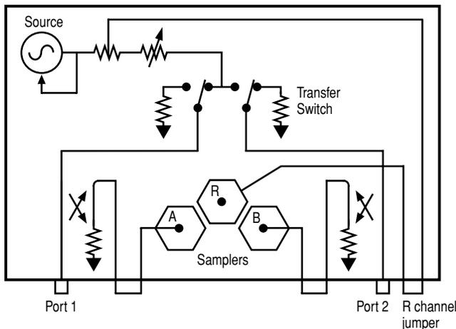
Option 400 and 012 test set block diagram
