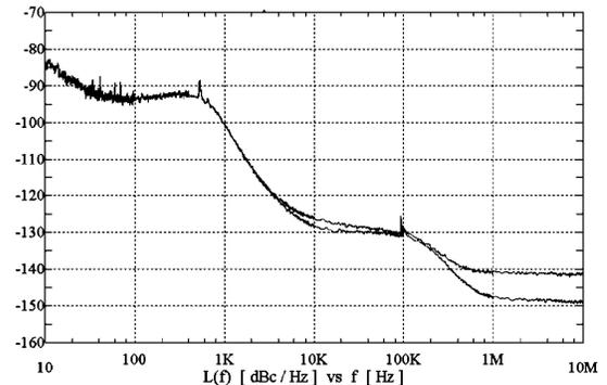
**fc = 1.8 GHz (CW and I/Q modulation on)**
