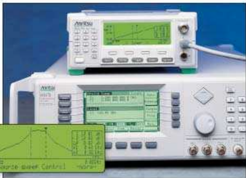
Source Sweep Graphic Display. Acquire power sweep or frequency sweep data at speeds greater than fifteen sweeps per second (GPIB to PC screen update rate). The meter automatically generates sweep synchronization with Anritsu 68000B or 69000A series Synthesized Sweep Generators.
