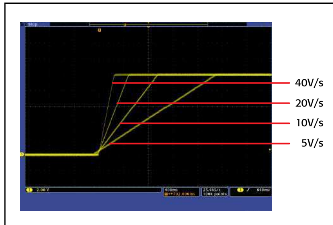
Precisely control voltage rise time with the variable slew rate control.
