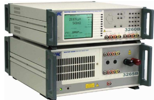
3265B/25A can deliver up to 25 A in steps of 25 mA
