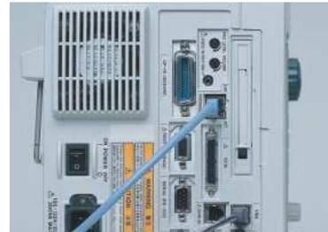
Just as for RS232 and GB-IB, you can write your own custom programs in Visual C++ 6.0 or Visual Basic 6.0 to control the DL750 through a USB interface.
