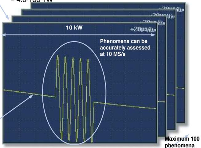
With DualCapture, the user sets triggers for capturing sudden phenomena. Up to 100 phenomena can be collected in a memory length of 10 kW at a maximum sampling rate of 10 MS/s.
